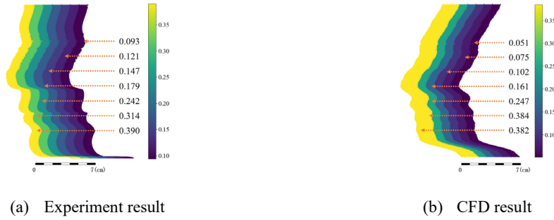
Fig.4 CFD Simulation Validation of the Airflow Visualization Experiment
